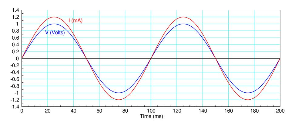
Voltage and current are in phase for resistors
