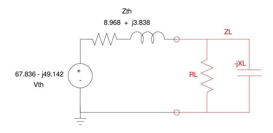
Solution: The load should be the complex conjugate of Zth
