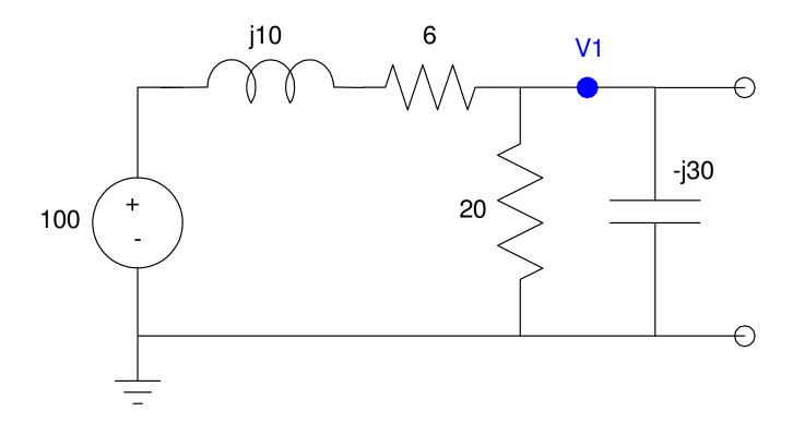
Solution: Combine the 20 Ohms and -j30 Ohms in parallel:
