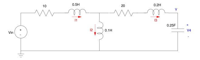
This problem is actually hard due to the constraint that I1 = I2 + I3. The problem is there isn't a capacitor at the middle node. So... add a capacitor there. Just make it small so it doesn't change much
