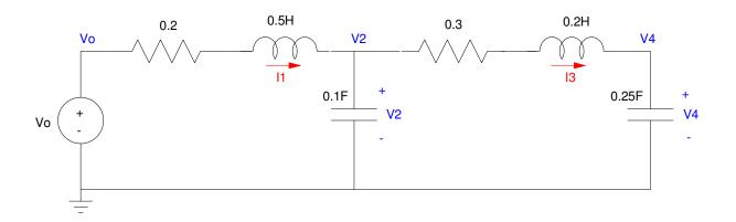
Step 1: Determine the initial conditions. Capacitors are open circuits at DC and inductors are shorts at DC. This results in
