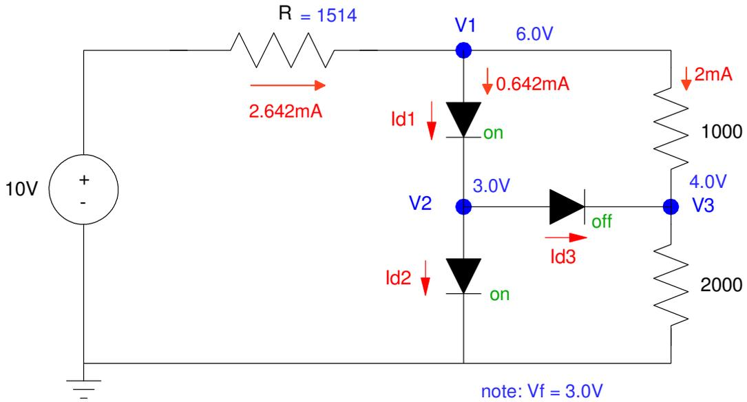
3) A green and white LED are connected to a 10V source. Determine the current and brightness of each LED.
