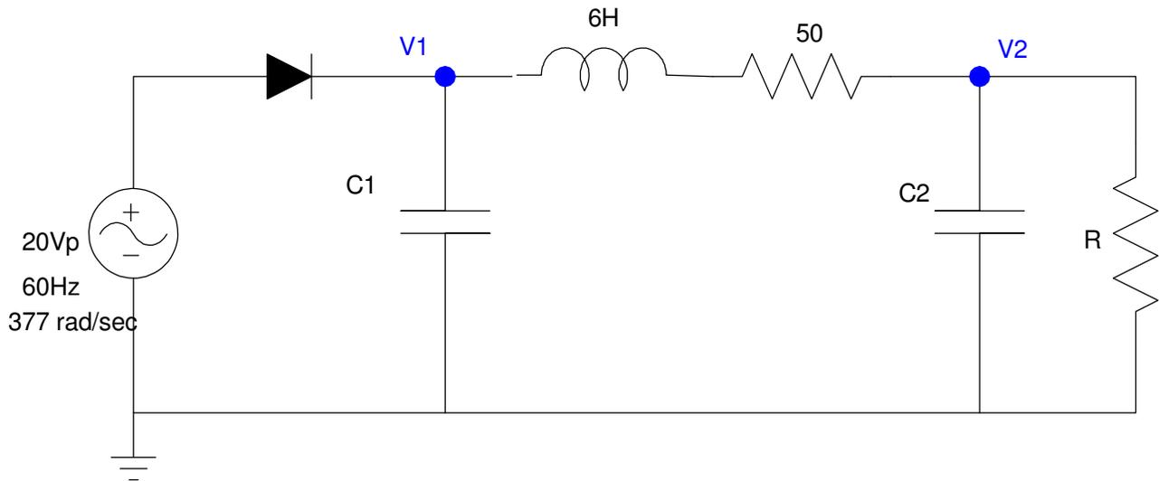
$$V_1(DC) = 19.3V - \frac{1}{2}(3V_{pp}) = 17.80V$$
