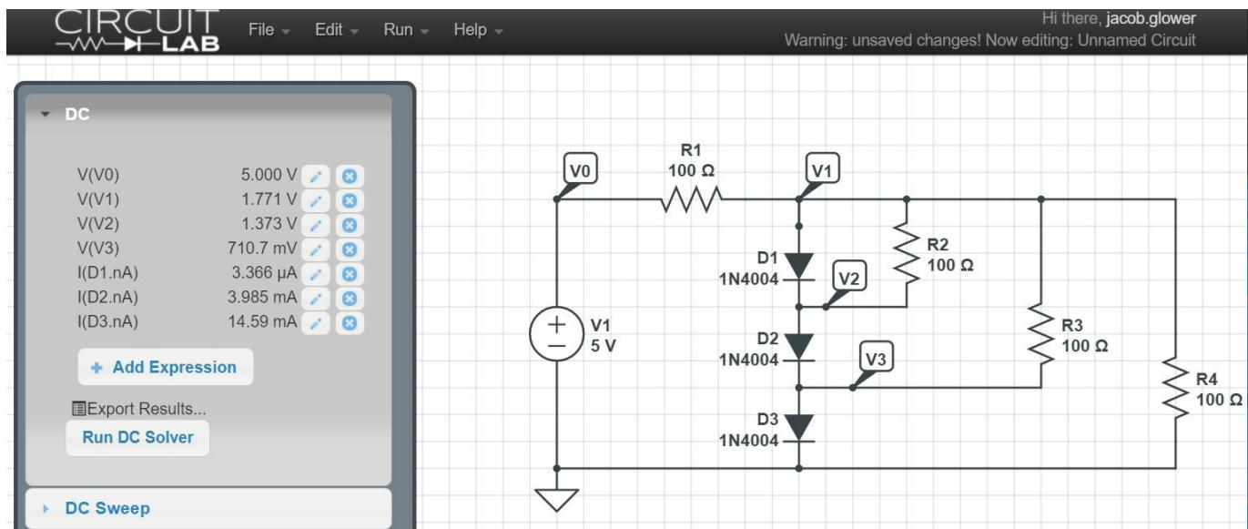
11) Build this circuit with your breadboard and measure {V1, V2, V3}
