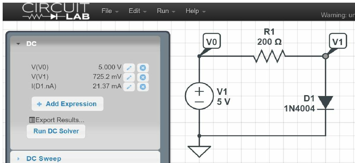
7) Build this circuit on your breadboard and measure Vd. From this, compute Id
