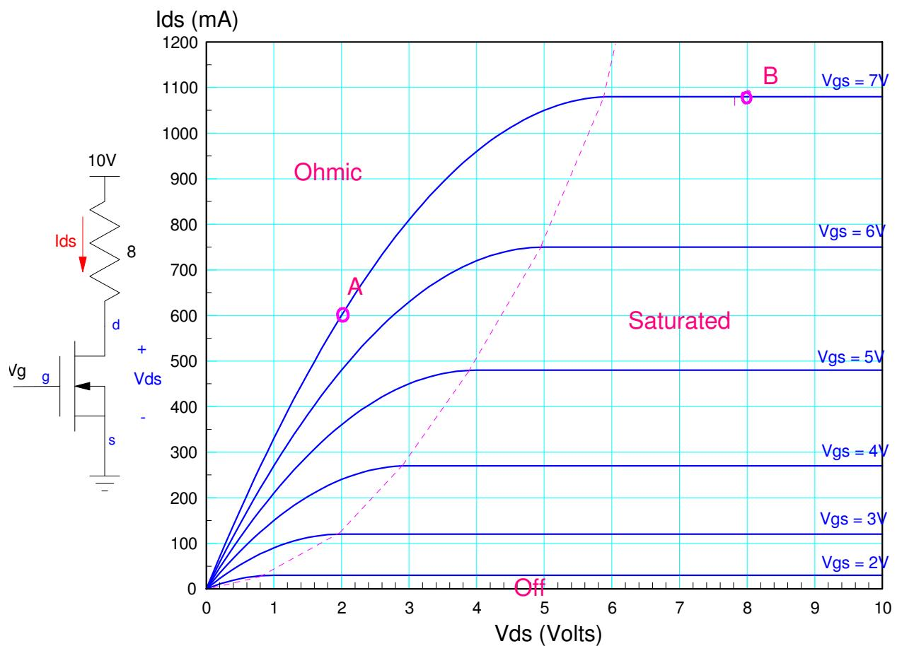
9) Draw the load line for the circuit below. From the load line, determine the operating point ( $V_{ds}$ ,  $I_{ds}$ ) when
