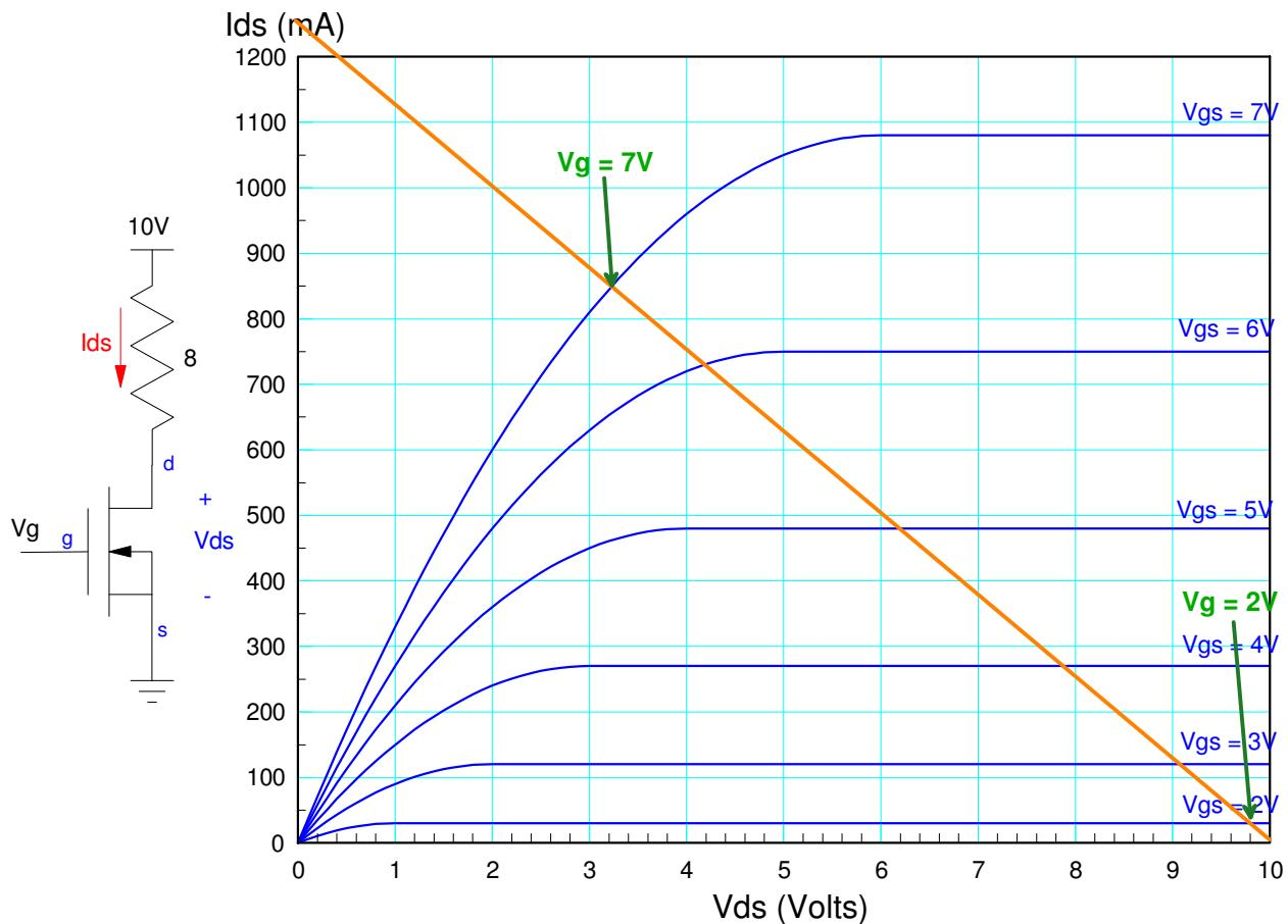
10) Calculate the operating point ( $V_{ds}$ ,  $I_{ds}$ ) when
