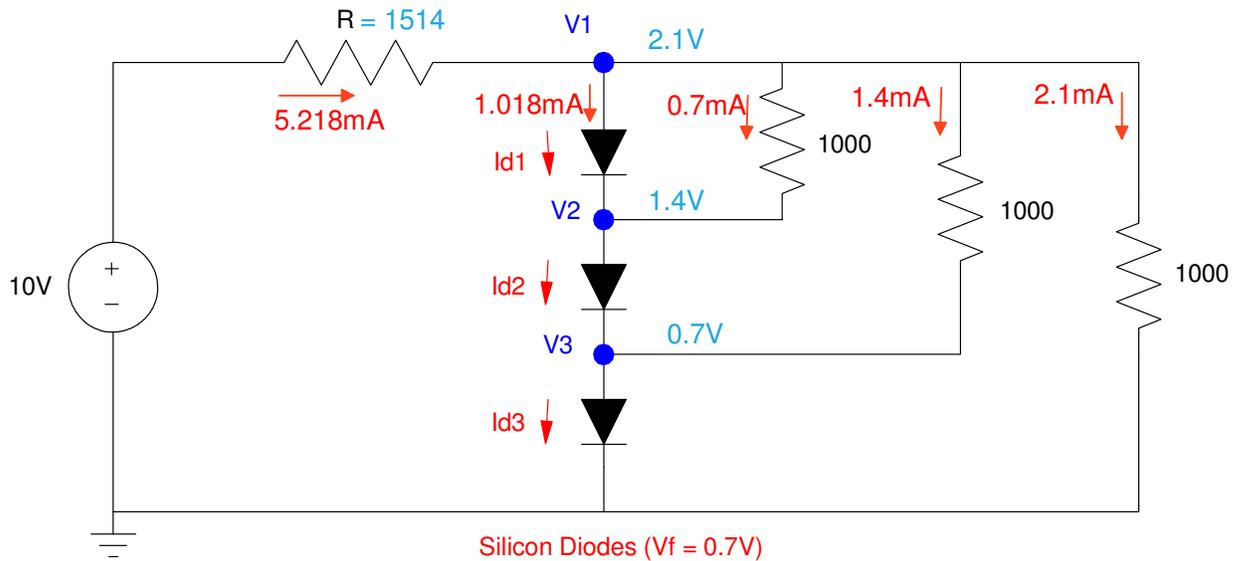
To find  $I_{d1}$ , do a voltage node equation at V1
