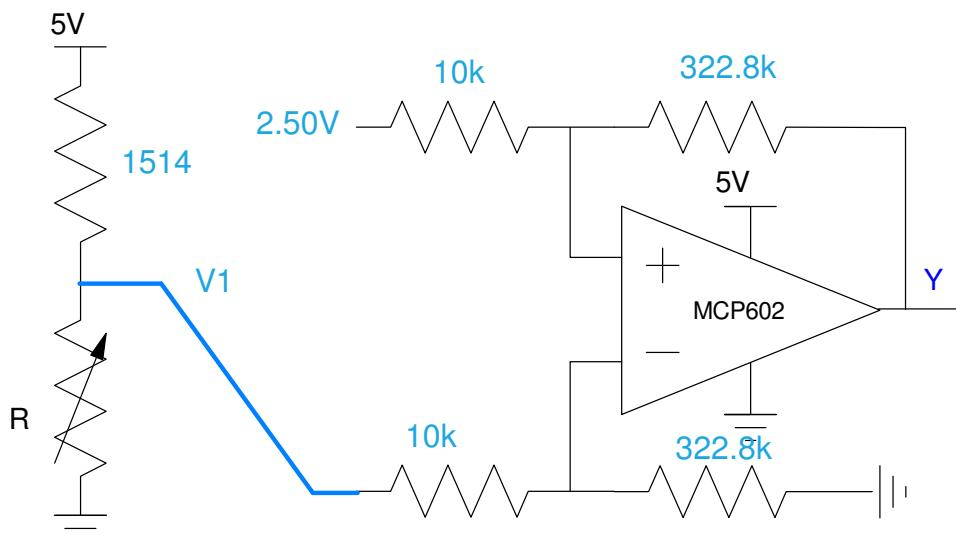
6) Schmitt Trigger: Analysis. Determine the voltages and resistance where the following Schmitt trigger turns on and off. Assume Rx is  $1000 + 100 \cdot (\text{Birth Month}) + (\text{Birth Day})$ . May 14th gives  $R_x = 1514$  Ohms.
