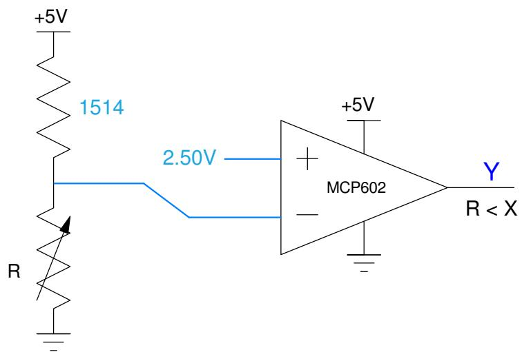
5) Schmitt Trigger: Design a circuit which output
