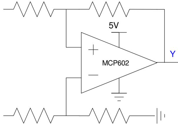
6) Schmitt Trigger: Analysis. Determine the voltages and resistance where the following Schmitt trigger turns on and off. Assume  $R_x$  is  $1000 + 10 * (\text{Birth Month}) + (\text{Birth Day})$ . May 14th gives  $R_x = 1514$  Ohms.
