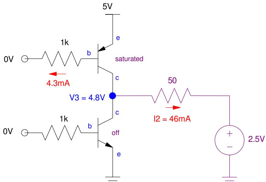
$0V : 0V$  results in  $V_2 = 4.8V$
