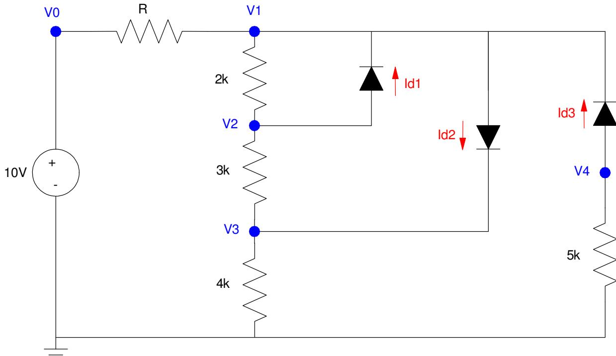
$$I_{d1} = 10^{-11} \cdot \left( \exp\left(\frac{V_2-V_1}{0.038}\right) - 1 \right)$$
