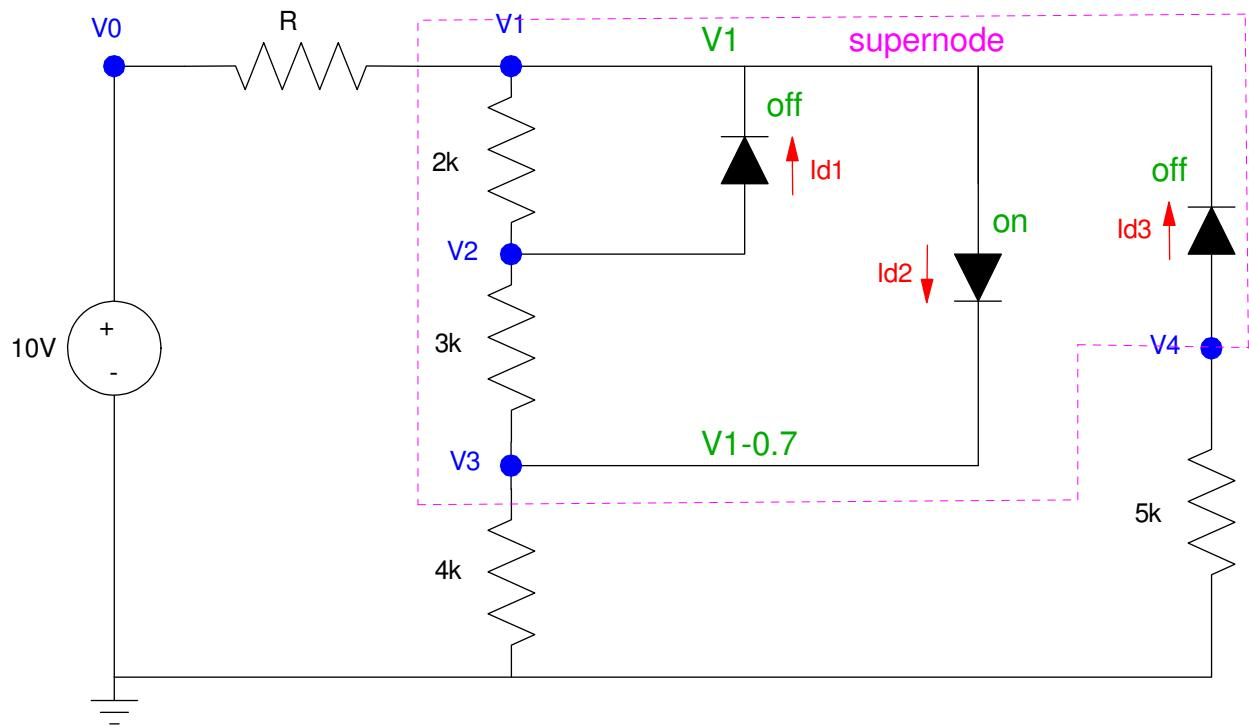
$$\left(\frac{V_1-10}{1414}\right) + \left(\frac{V_1-0.7}{4k}\right) + 0 = 0$$
