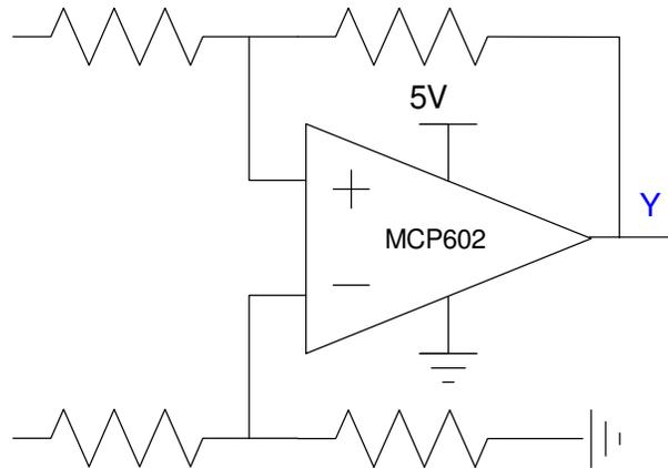
6) Schmitt Trigger: Analysis. Determine the voltages and resistance where the following Schmitt trigger turns on and off. Assume  $R_x$  is  $900 + 10 * (\text{Birth Month}) + (\text{Birth Day})$ .
