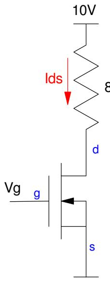
5) Simulate this circuit in CircuitLab using an IRF3710. Determine the voltages and currents when
