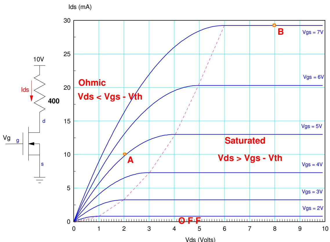
2) Draw the load-line for the circuit below. From the load line, determine the Q-point ( $V_{ds}$ ,  $I_{ds}$ ) when
