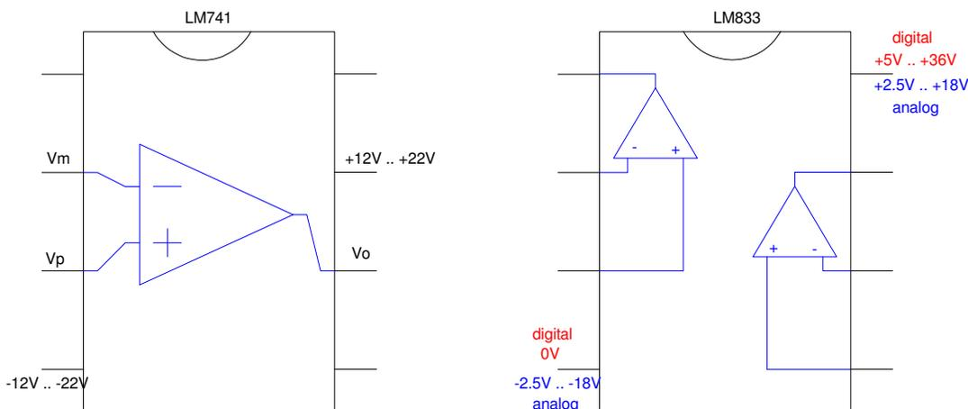
Pin Layout for two common op-amps: LM741 and LM833
