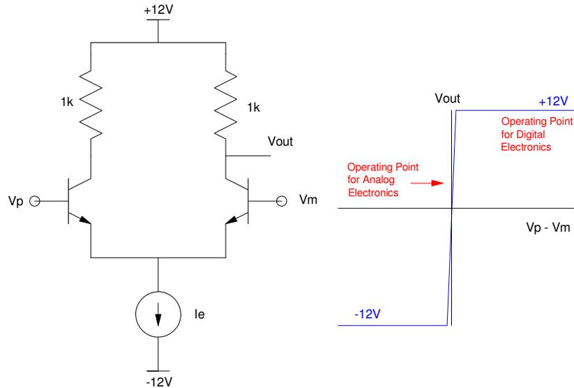
In ECE 320, we wanted binary outputs: a motor is either 100% on or 0% on (i.e. off). Likewise, we operated the transistors at the rails: either  $+5V$  for logic 1 or  $0V$  for logic 0. Towards this end, the transistors we used were always off or saturated.
