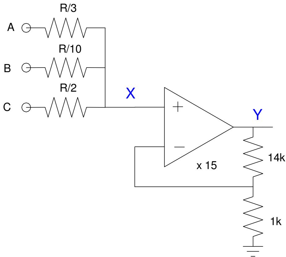
3) Determine Y as a function of A, B, and C. Assume ideal op-amps
