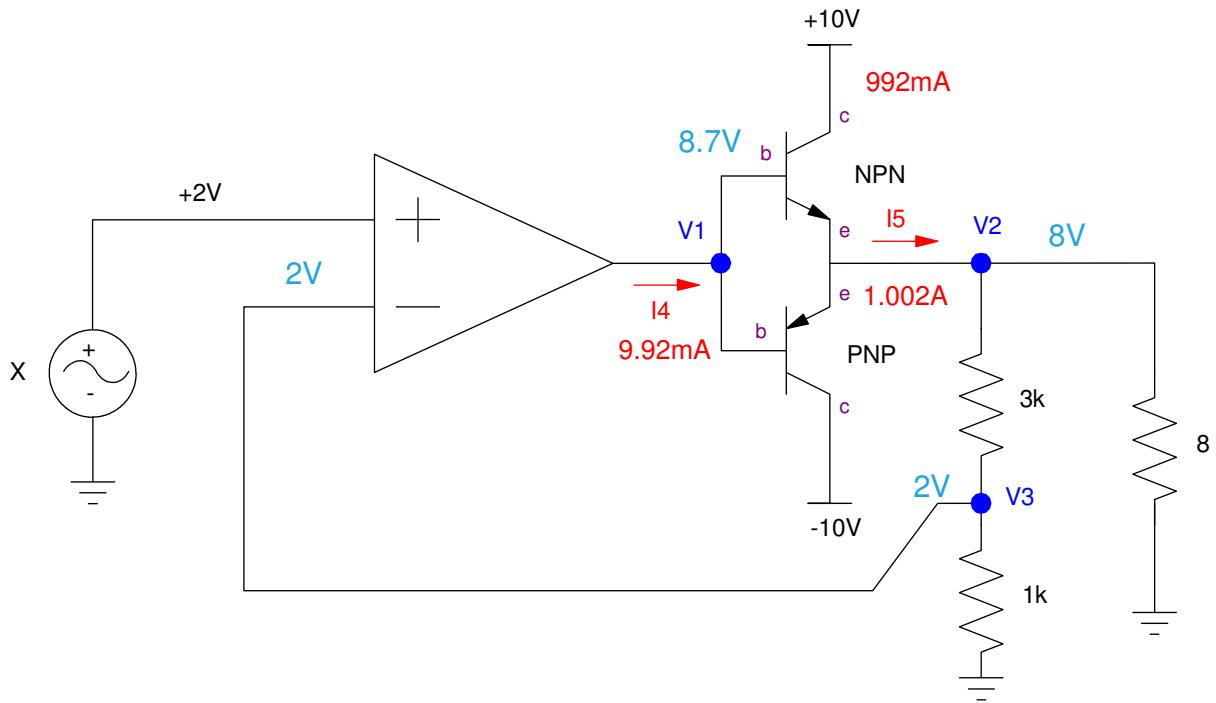
6) Determine the voltages for the following push-pull amplifier. Assume
