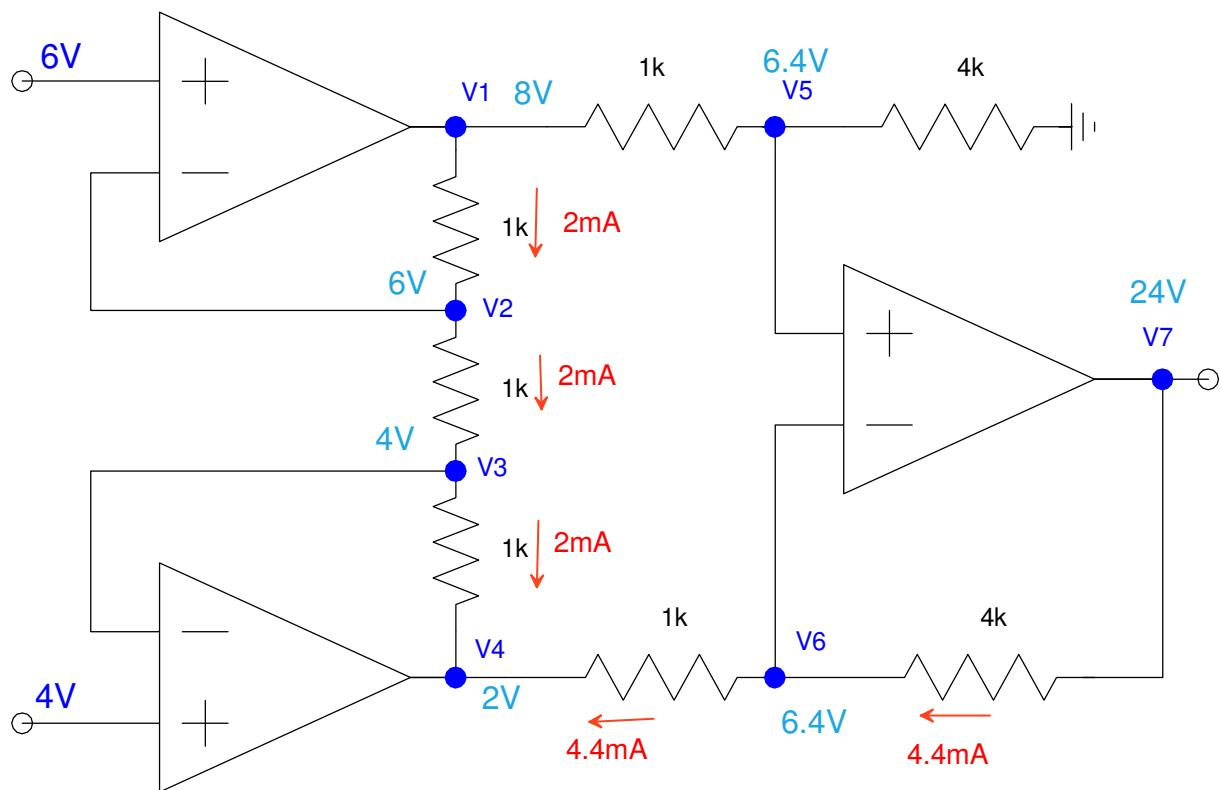
5) Determine the voltages for the following push-pull amplifier. Assume
