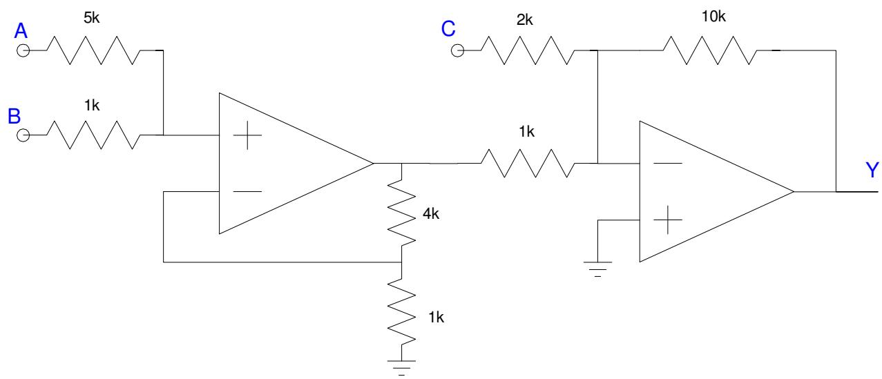
4) Determine the voltges for the following op-amp circuit. Assume ideal op-amps
