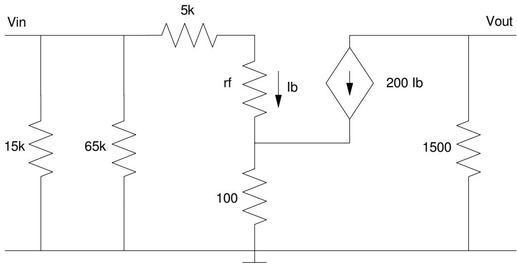
4) Determine the 2-port model for the following circuit
