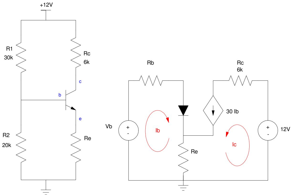
**6. 2-Port model:** Determine the 2-port parameters for the following circuit. Assume
