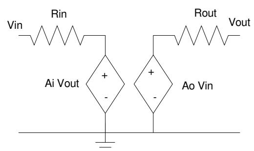
**7. 2-Port model:** Determine the 2-port parameters for the following circuit. Assume
