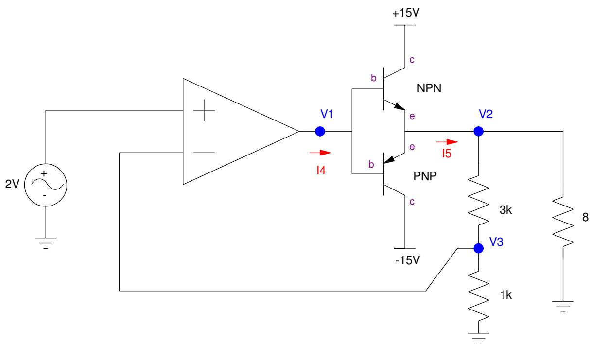
5) Determine the voltages for the following push-pull amplifier. Assume TIP transistors
