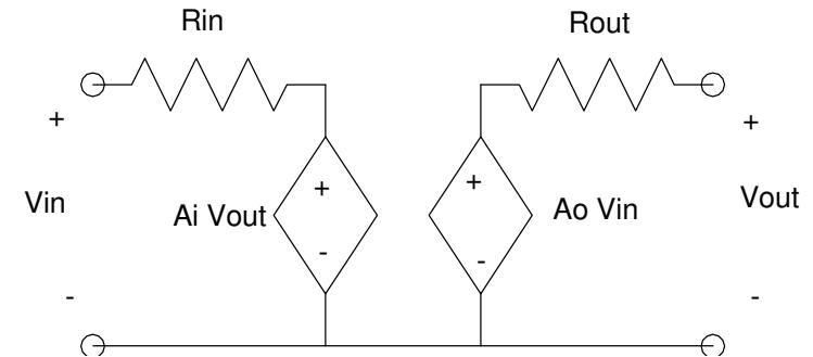
**R<sub>out</sub>:** For the 2-port model, short V<sub>i</sub> so that V<sub>i</sub>=0 and  $A_o V_{in} = 0$ . Measure the resistance at the output. Doing the same for the CE amplifier, this results in
