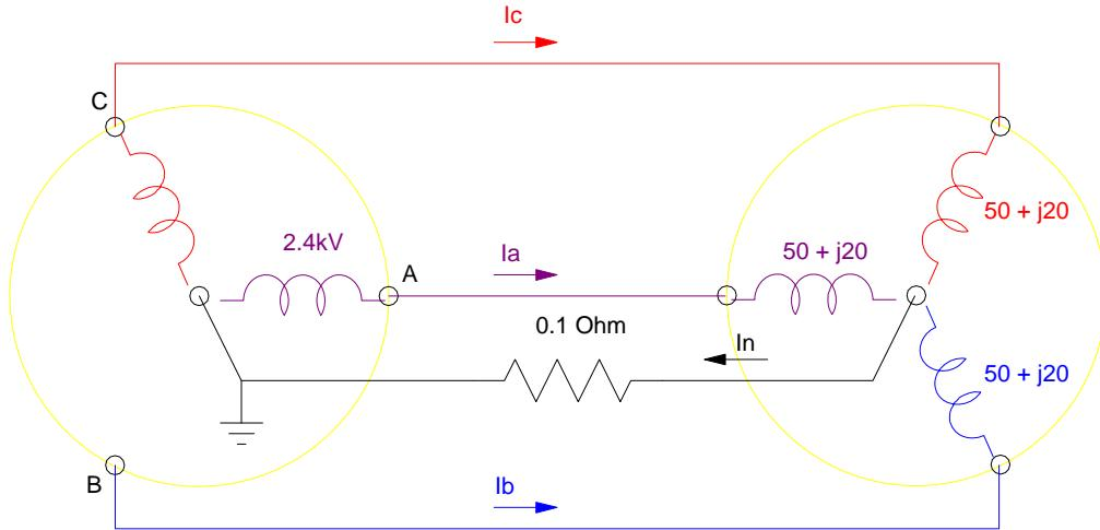
To model the loss of phase B, add 1G Ohm impedance to line B:
