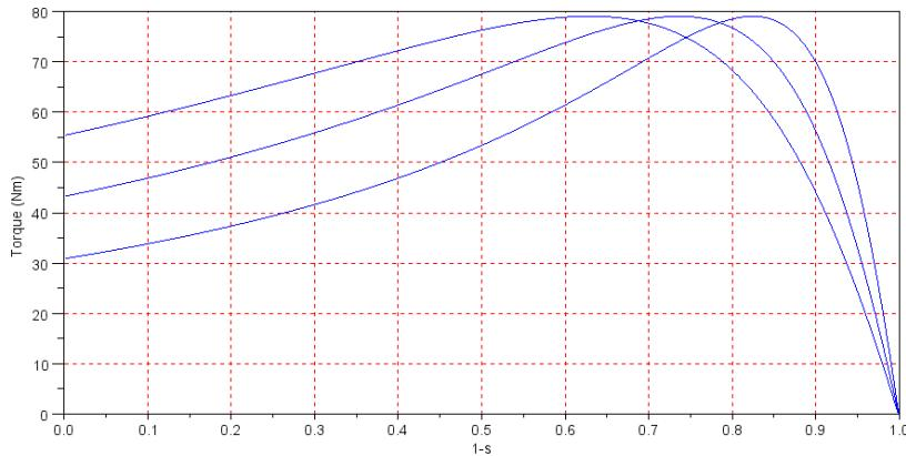
$r_2 = 0.1$  (bottom curve),  $0.15$ ,  $0.2112$  (top curve)
