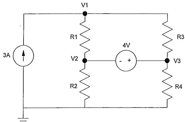
$$-3 + \frac{V_1 - V_2}{R_1} + \frac{V_2 - V_3}{R_2} = 0$$
