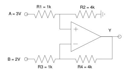
Homework #7, problem #3. Find the pdf for the voltage at Y. All resistors are 5% tolerance
