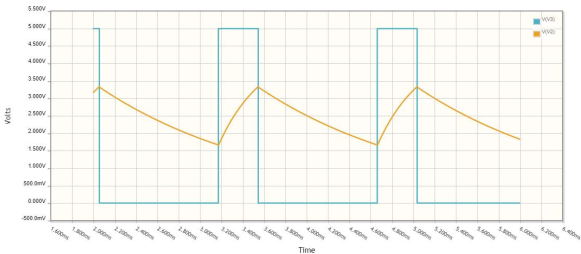
Resulting Voltages: The period is 1.486ms and the duty cycle is 25.2%
