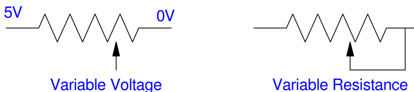
Two common configurations for potentiometers
