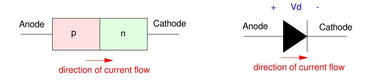
Symbol for a diode: Diodes only allow current to flow from the anode to the cathode
