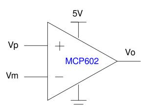
The MCP602 is a high-gain differential amplifier, where
