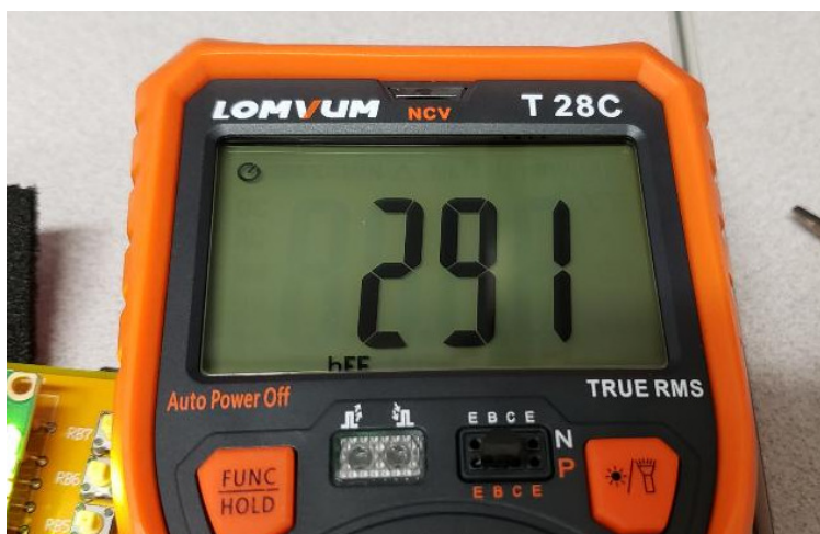
Measuring the gain of a PNP transistor: hfe = 291
