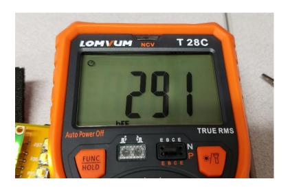
For example, measuring the gain of several 3906 PNP transistors results in
