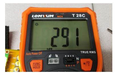
For example, measuring the gain of several 3906 PNP transistors results in
