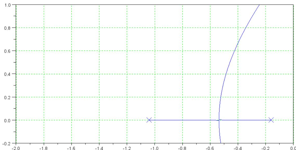
Determine the design point (s at the breakaway point)
