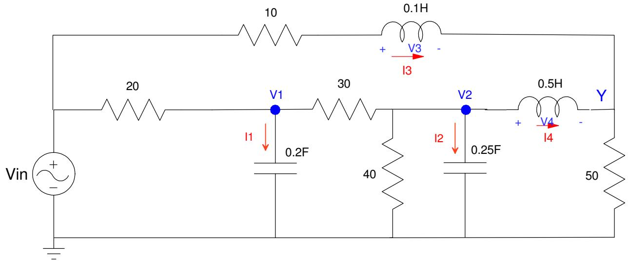
$$I_1 = 0.2sV_1 = \left( \frac{V_{in} - V_1}{20} \right) - \left( \frac{V_1 - V_2}{30} \right)$$
