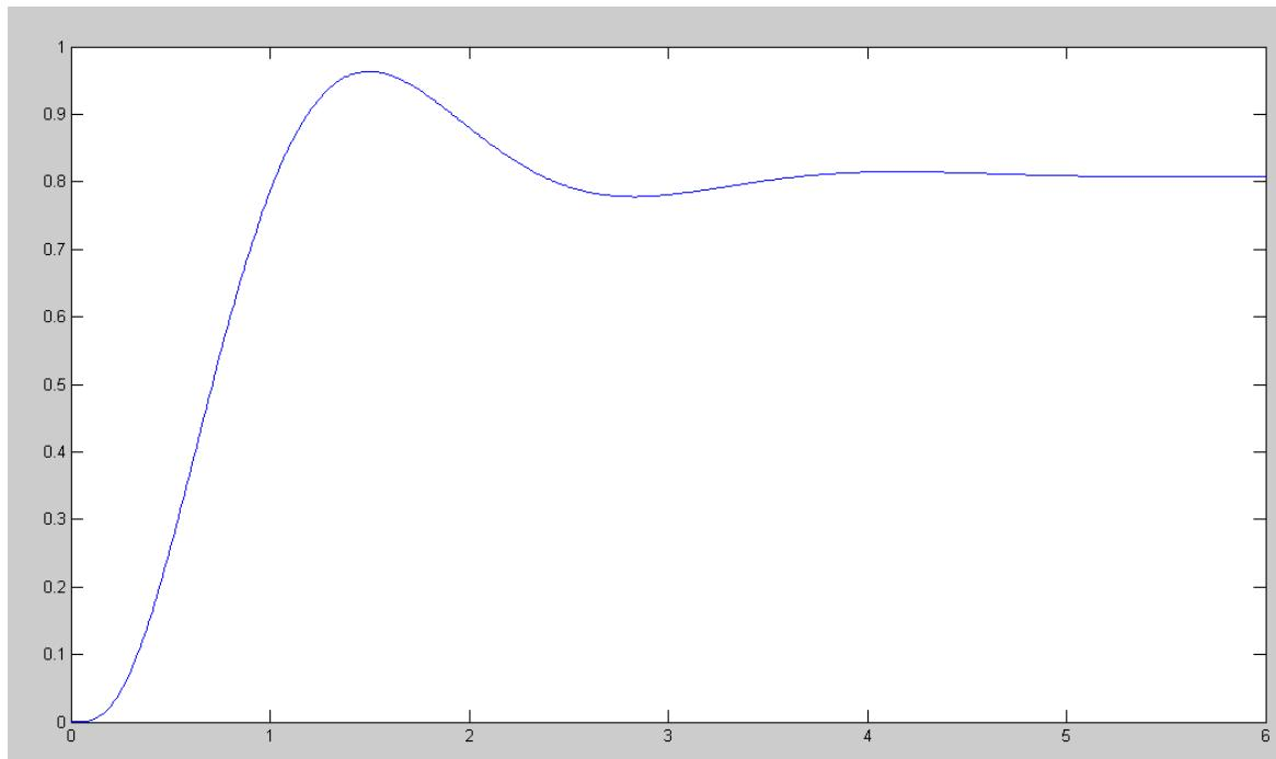
3) Design a lead compensator,  $K(s) = k \left( \frac{s+a}{s+10a} \right)$ , which results in 20% overshoot for a step input.
