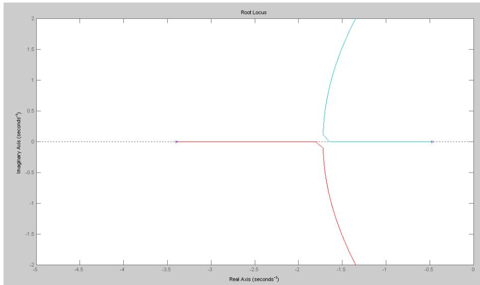
Step 2: Pick a point on the root locus. Since we want the fastest system with no overshoot, pick the breakaway point
