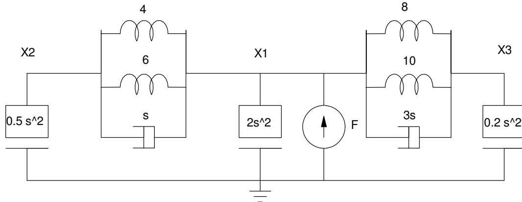
Write the equations of motion (i.e. write the voltage node equations)
