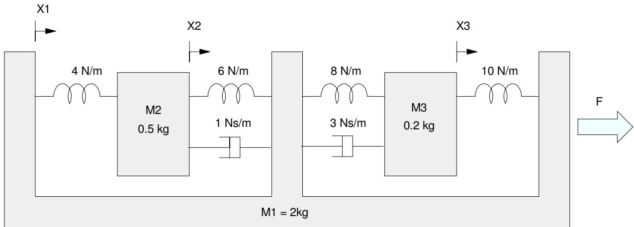
Draw the circuit equivalent for the following mass-spring system
