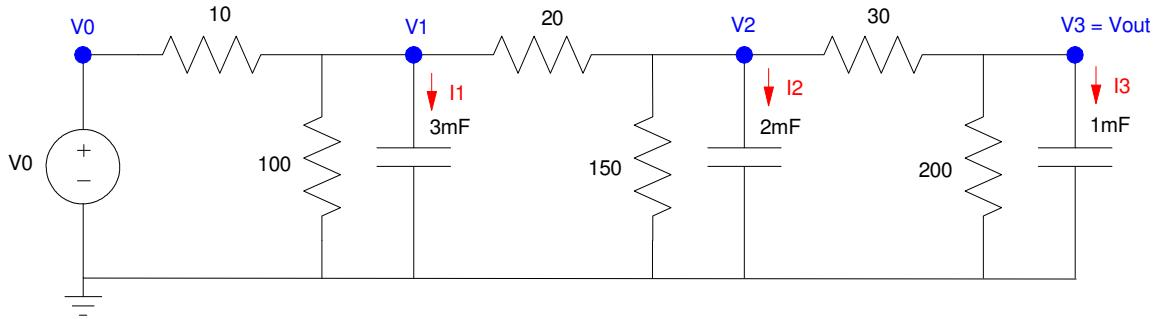
$$I_1 = C_1 s V_1 = \left( \frac{V_0 - V_1}{10} \right) + \left( \frac{V_2 - V_1}{20} \right) + \left( \frac{0 - V_1}{100} \right)$$
