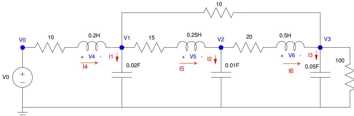
Use the currents in the inductors and voltages across the resistors as the energy states
