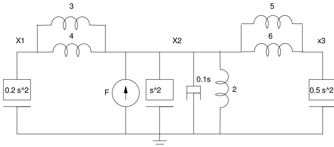
Step 2: Write the voltage node equations
