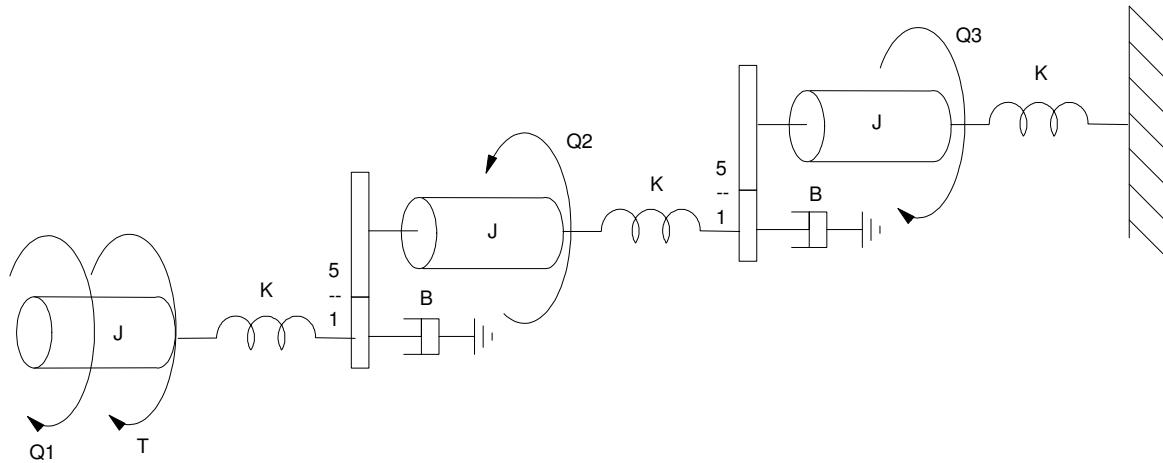
Problem 3:  $J = 0.2 \text{ Kg m} / \text{s}^2$ ,  $B = 0.1 \text{ Ns/m}$ ,  $K = 5 \text{ Nm/rad}$
