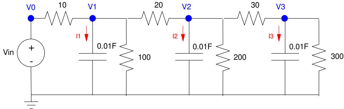
$$I_1 = CsV_1 = \left( \frac{V_0 - V_1}{10} \right) + \left( \frac{V_2 - V_1}{20} \right) - \left( \frac{V_1}{100} \right)$$
