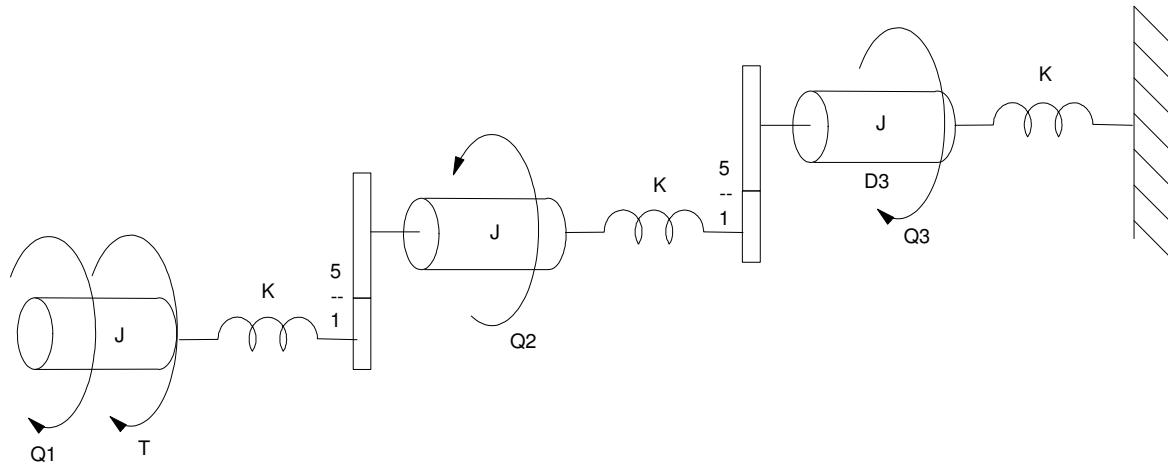
Problem 3:  $J = 2.5 \text{ Kg m} / \text{s}^2$ ,  $K = 20 \text{ Nm/rad}$ ,  $D_3 = 1.5 \text{ Nms/ rad}$
