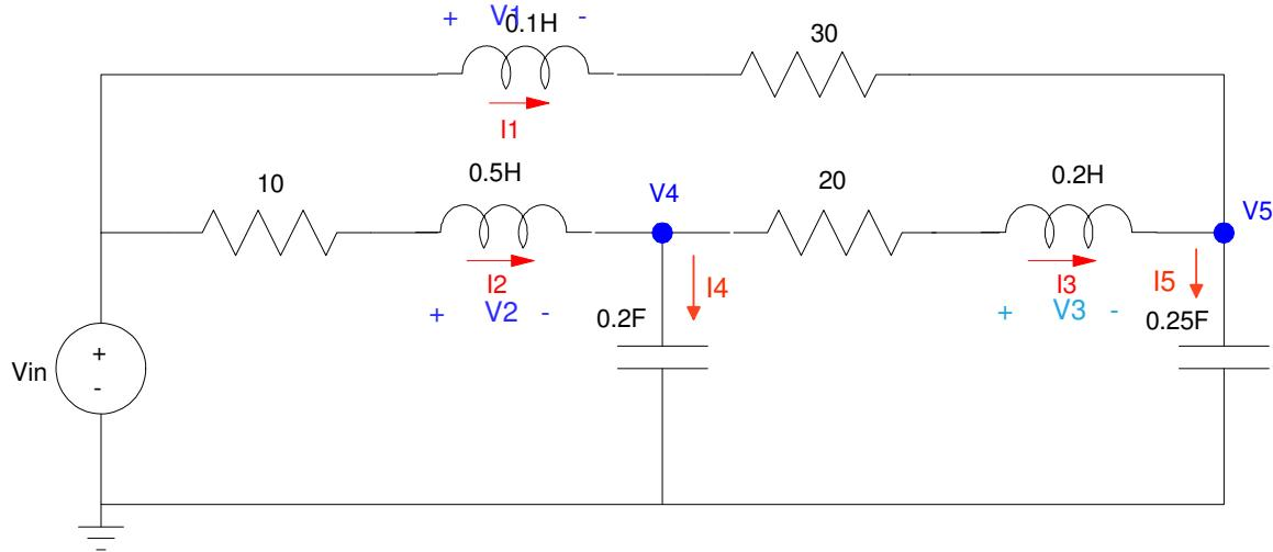
The energy in the system is defined by the current in the inductors and the voltage across the capacitors.
