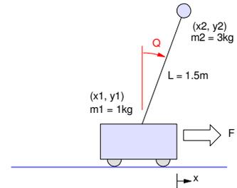
Design a control law so that the cart and pendulum system behaves like the following reference model:
