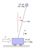
Design a control law so that the cart and pendulum system behaves like the following reference model:
