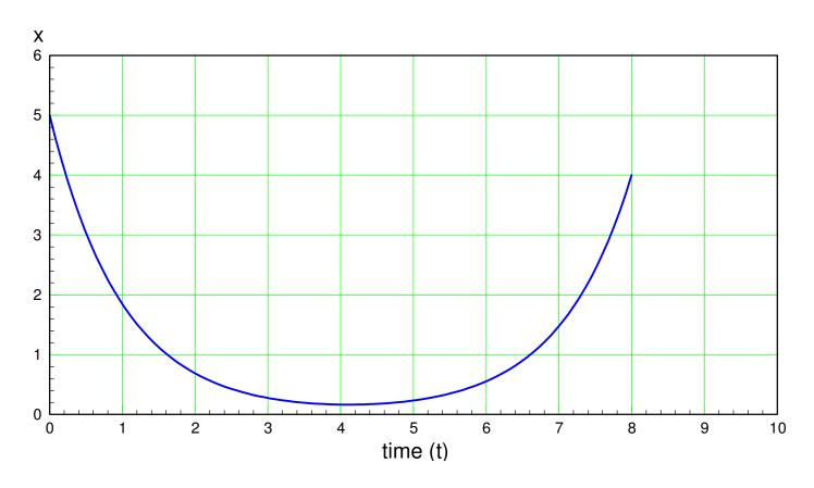
Optimal path of x(t) with the cost function  $J = \int_0^1 (x^2 + \dot{x}^2) dt$
