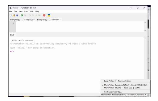
Once Thonny is installed, connect your Pico board to the computer then click on the lower-right corner to install MicroPython
