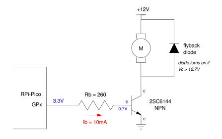
This limits the voltage at Vc to +12.7V
