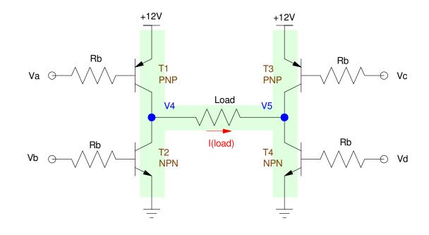
note: Each transistor has a slight voltage drop (Vce) when saturated - resulting in the load sseeing slightly less than +/- 12V when turned on
