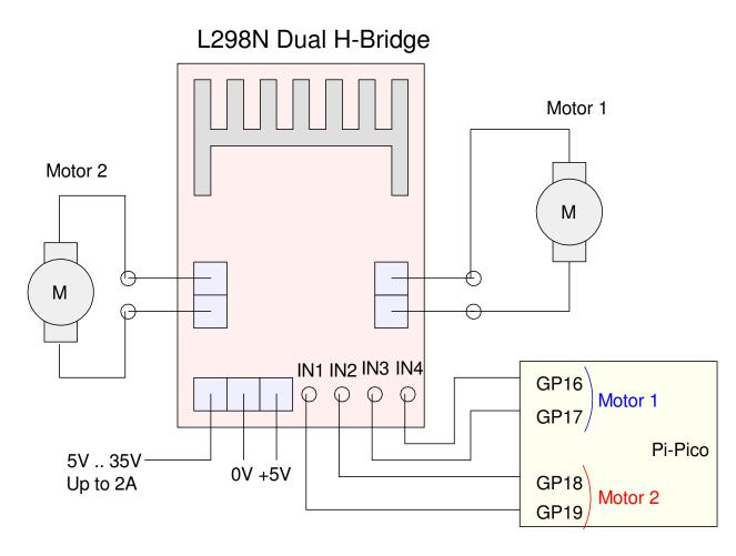
Two DC motors can be driven with a dual H-bridge driver
