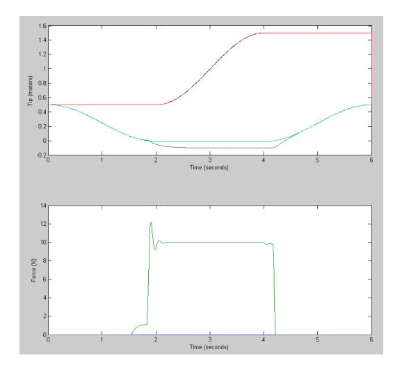
Resulting tip position and tip force. Note that while in contact the tip force is held at 10N as desired.
