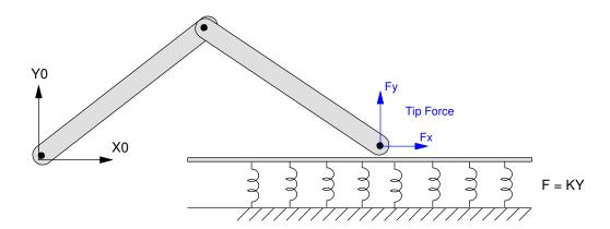
Now, the tip is allowed to go below zero - sinking into the floor slightly. When it does so, a tip force results, opposing the robot. This tip force then translates to the joint torques through the Jacobian as
