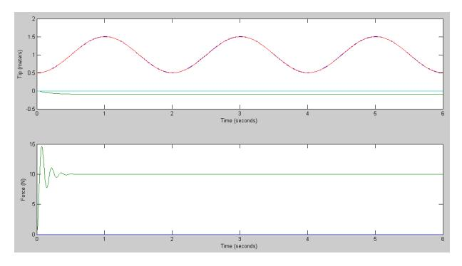
Resulting tip position and tip force. The tip force is regulated at 10N as desired.
