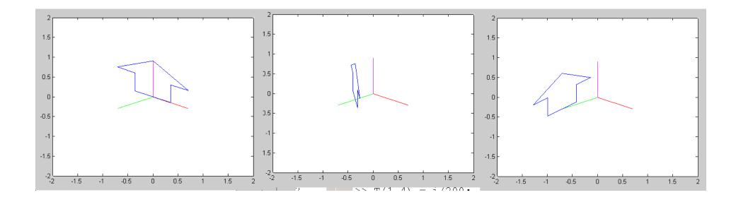
The arrow spins about its Z-axis (Tz) while translating along the x-axis
