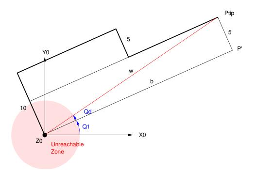
From this point on, the previous equations all apply, with the note that 'b' is the value computed here rather than the distance to the tip (called 'w' here)
