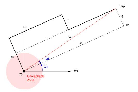
Top View of the PUMA Robot. The shoulder and elbow offsets do not cancel, resulting in a 5cm offset for the tip
