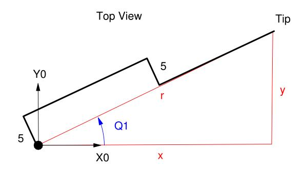
Top View of the RRR robot. Note that the two offsets cancel resulting in Q1 point to the tip.
